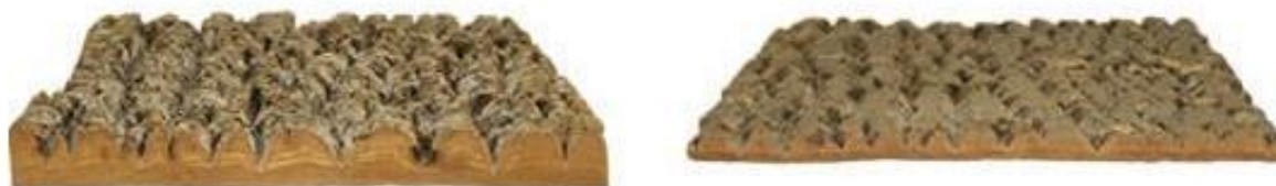
Figure 12. Example of two different grades of poplar bark panels
