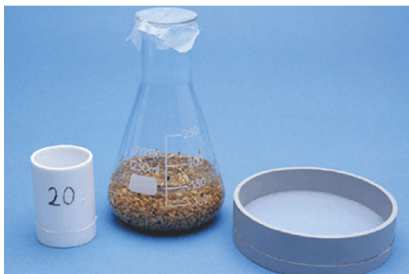
Fig. 10 Size-selective sieving wash test: 20 µm mesh nylon sieve (mounted between 4-cm diameter cylinders, left), 53-µm sieve (mounted between 11-cm diameter cylinders, right) and a 50-g grain sample in a 250-mL Erlenmeyer flask with 100 mL of 0.01% Tween-20 aqueous solution.
