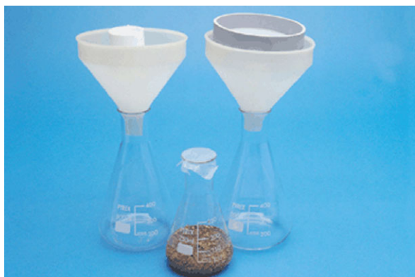
Fig. 11 Size-selective sieving wash test: arrangement of sieves (20-µm sieve, left; 53-µm sieve, right) mounted in funnels over 500-mL Erlenmeyer flasks in preparation for size-selective sieving of wash water from a 50-g grain sample.
