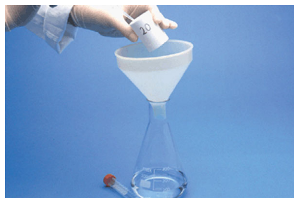
Fig. 13 Size-selective sieving wash test: the final sieve fraction being washed to one side of the 20-µm sieve with water from a disposable Pasteur pipette in preparation for recovery.
