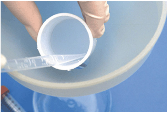
Fig. 14 Size-selective sieving wash test: the final sieve fraction being recovered from the 20- \mu\text{m} sieve with water from a disposable Pasteur pipette for subsequent centrifugation in a conical centrifuge tube.
