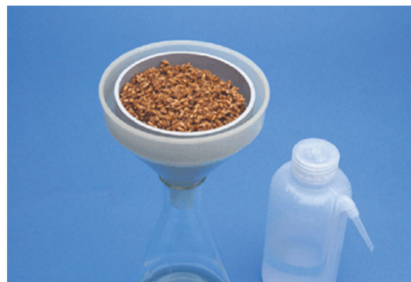
Fig. 12 Size-selective sieving wash test: grain and washings poured onto a 53-µm sieve over a 500-mL Erlenmeyer flask, together with an aspirator bottle for subsequent rinsing of the grain on the sieve.
