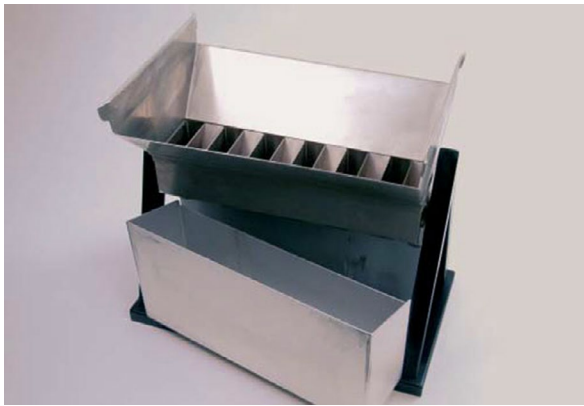
FIGURE 2 Example of a riffle sampler [Colour figure can be viewed at wileyonlinelibrary.com]
