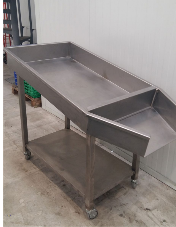
FIGURE 1 Example of a specific inspection table. (Courtesy: Vañó García.)
