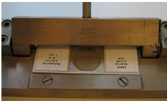
FIGURE 4 Labels added and sides of aluminium slide used to secure sealed coverslips. (Courtesy: NRC-PPPO, NL.)
