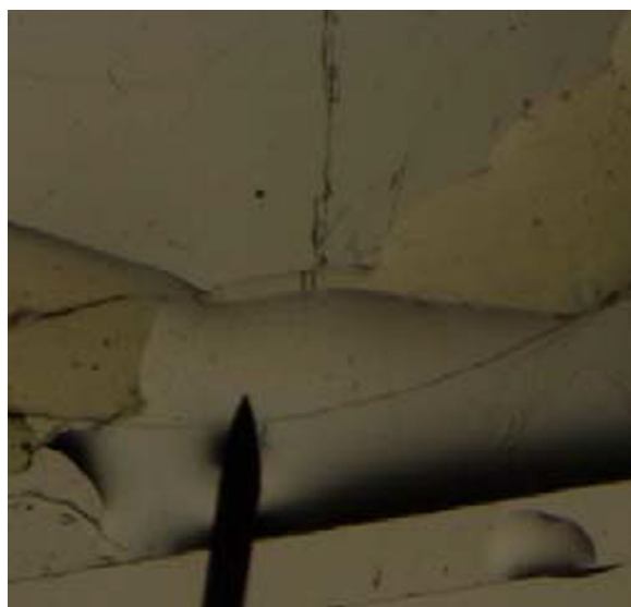
FIGURE 44 Coverslip lifted with a hypodermic needle to encourage infusion of glycerol. (Courtesy: Fera Science Ltd, GB.)
