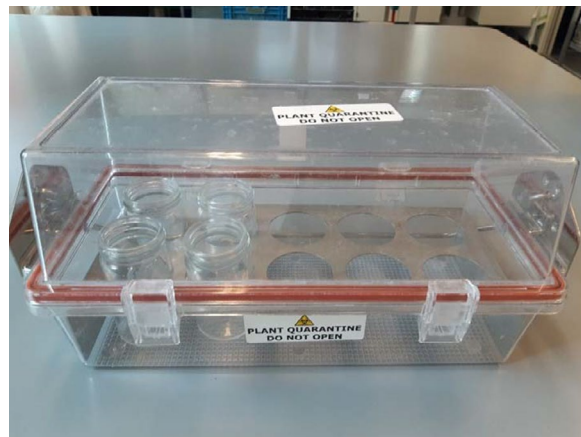
FIGURE 31 Biosafety transport box with nematode suspensions in glass jars. (Courtesy: NRC-NPPO, NL.)
