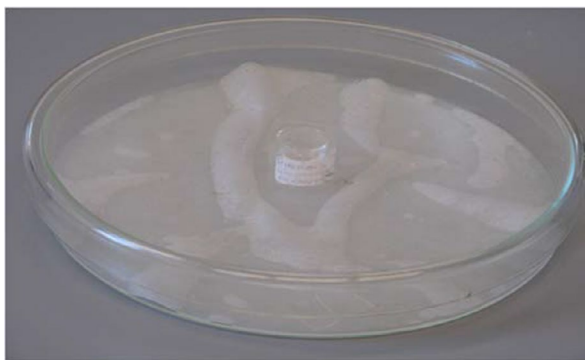
FIGURE 37 Specimens in solution on a filter paper infused with glycerol. (Courtesy: NRC-PPPO, NL.)
