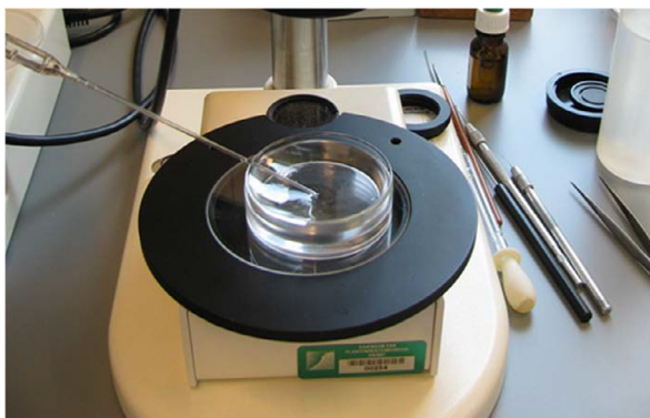
FIGURE 35 Excess 70°C TAF added to nematodes suspended in a small drop of water. Nematodes are placed in a small amount of water, to allow rapid mixing with the fixative. TAF heated to 70°C is added in excess to the water droplet. The combination of killing and fixing the nematodes in one step results in reduced shrinking of nematodes. (Courtesy: NRC-NPPO, NL.)
