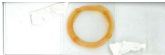
FIGURE 38 Coverslips on a Cobb slide removed and secured to a glass slide. (Courtesy: Fera Science Ltd, GB.)
